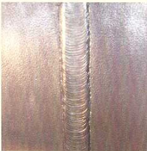
Performed Weld By GMAW Method
